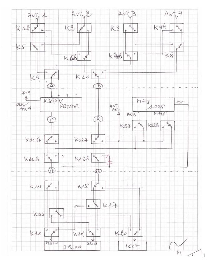
The four Rx Ant. inputs are addressed into two inner lines "A" and "B" which pass through two separate KD9SV preamplifiers (and Front End Savers) and can be switched to each of the three receivers. The MFJ 1025 can also be inserted and the inputs easily swapped from the front panel from one line to another, or to a 5<sup>th</sup> dedicated noise antenna, to try the best phasing opportunity between several antennas without the need to plug or unplug any coax connector.
