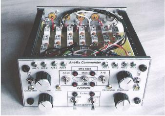
The Ant-Rx Combiner selects also which antenna group is going to be switched in the Rx.Ant.Switching Box for the desired direction. So only one flip is needed to change antennas or directions.
