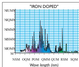
The standard 360 NM lamps used to cure transparent lacquer can be interchanged with 420 NM lamps suitable for coloured paints.
