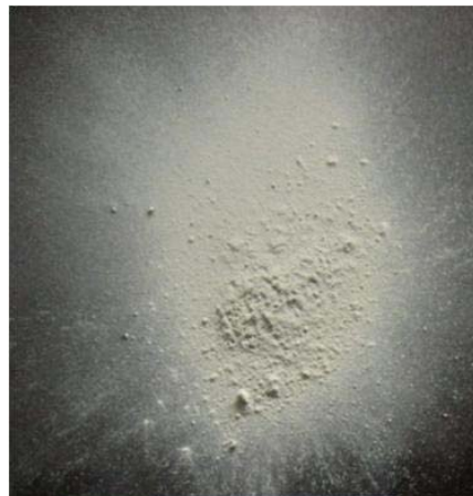
Dry mortar without ARBOCEL
