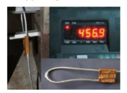
Test result, NOT cut the NPC wire
