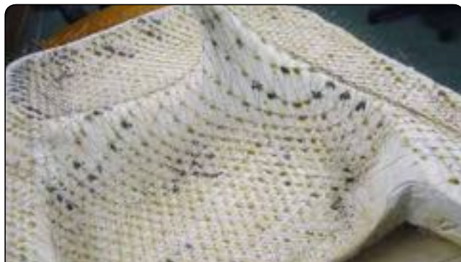
Plaster mold to form the steel wire structure
