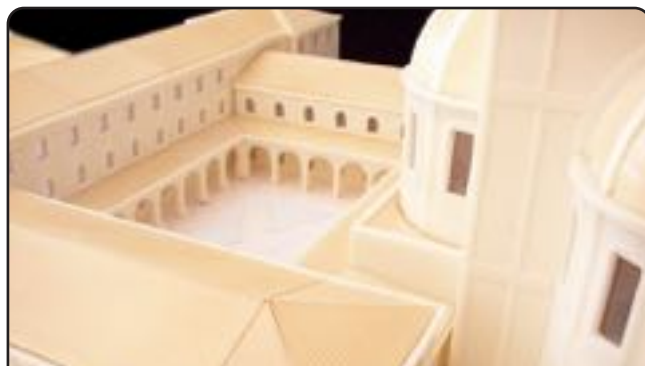
Repetitive elements such as the courtyard portico were created with a single mould
