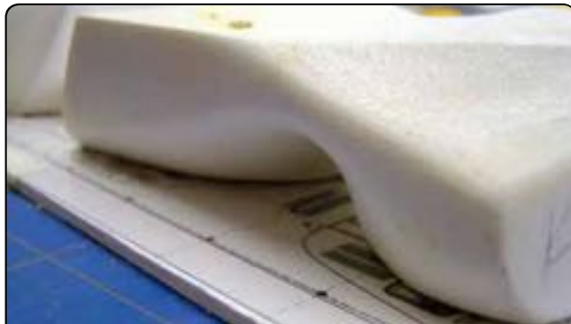
Epoxy resin copy of the original shape in foam handmade
