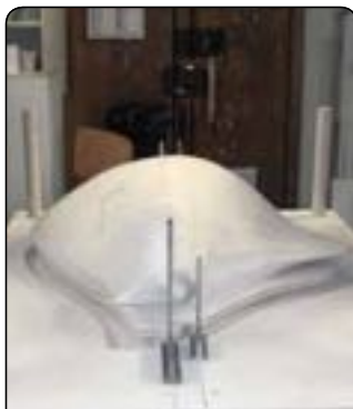
Solid shape to thermoforming the skin
