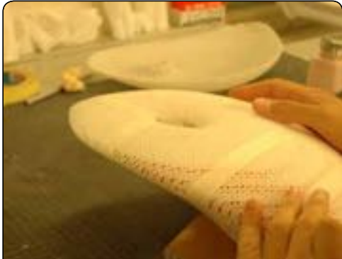
1.200 Scale model detail of 3D printed mesh
