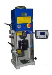
Gamma press T-25 is a machine designed for crimping wire sizes up to 10 sqmm.
