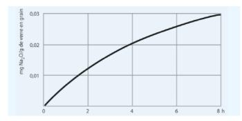
Hydrolytic attack on DURAN® as a function of time (100 °C)
