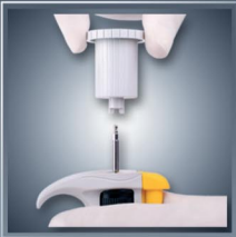
Insert calibration key and locate in key slots. The calibration key is delivered with the pipette.
