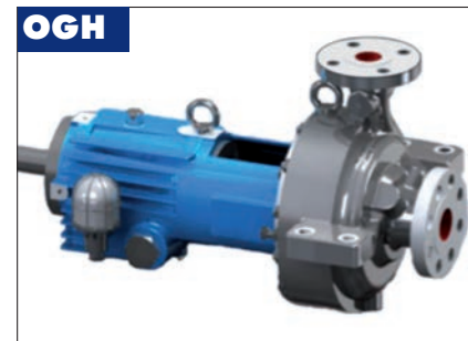
RADIAL SINGLE IMPELLER CENTRIFUGAL PUMP “OGH” WITH HORIZONTAL SHAFT, DESIGNED ACCORDING TO API 610 12 th EDITION CATEGORY OH2, SUITABLE FOR HEAVY PROCESS INDUSTRY, Oil&Gas, POWER PLANTS, OFFSHORE AND SPECIAL FIRE-FIGHTING SYSTEMS.
