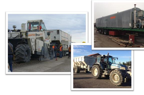
In cold recycling, the existing road pavement structure is milled. By adding binders, a new compound of building materials is formed which is directly re-applied by the stabilizer and which serves as a load-bearing or foundation layer. With this method, 100% of both coherent and inconsistent layers are reused.
