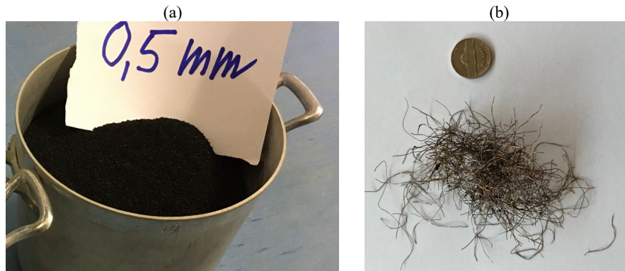
Fig. 1. Tire recycled materials used in the cement-based mortars: (a) rubber granulates (sieve residue at a 0.5 mm); (b) recycled steel fibers (average length 34 mm).
