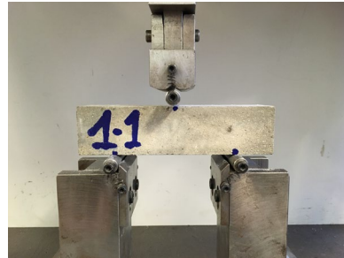
Fig. 2. The three-point bending tests of cement-based prisms (UNI 196-1 [7]).
