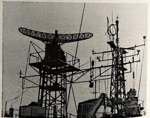
Selenia SF-1 search radar antenna on the Royal Danish Navy 'Falster' class minelayer, Sjelland. Bottom right can be seen the Contraves Sea Hunter FCS radar group. (Stefan Terzibaschtsch)
