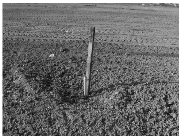
Fig. 1. View of a piezometer used for in situ gas monitoring.
