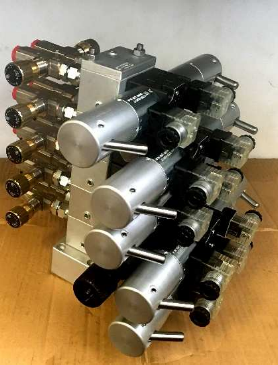
Manifold with valve's backup leverage
