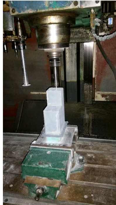
Autoclave consolidation and CNC machining
