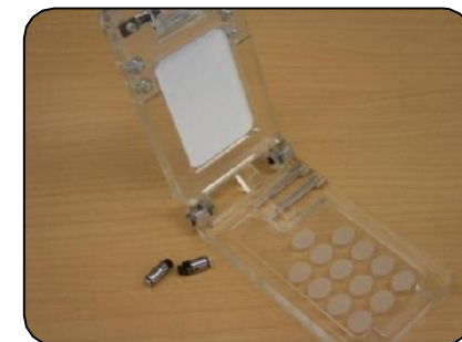
Hold type hinge in “flip” phone headset.
