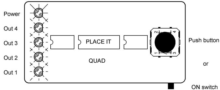
If the IC is in good condition: Flash LED 1 , LED 2 , LED 3 , LED 4
