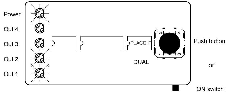
If the IC is in good condition: Flash LED 1 e LED 2
