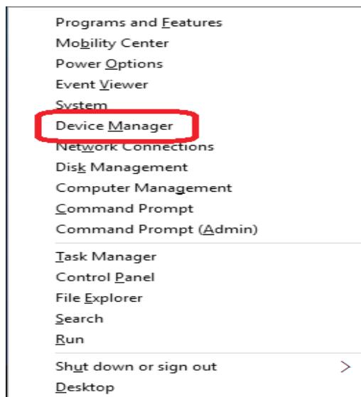
Open Device Manager and under the item Ports (COM and LPT) locate the item of the virtual serial port "Roottech CH340" or "USB to Serial CH340" next to it the corresponding serial port number will be indicated.
