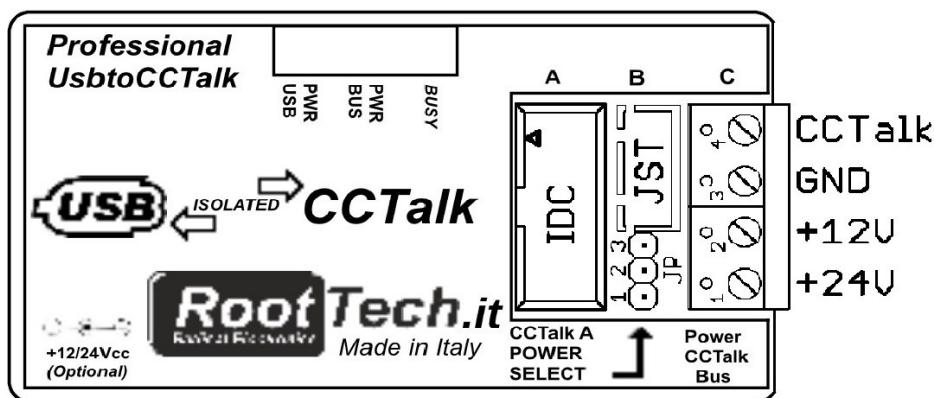
The interface is equipped with the standard connectors most used in CCTalk peripherals, however the **CCTalk BUS** is available at **PIN4** of the terminal block , in order to be able to wire a possible CCTalk HUB or a peripheral with a connector not standard or not present on the interface.
