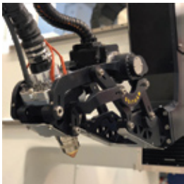
2 TESTA BEVEL PLASMA PLASMA HEAD WITH BEVEL SYSTEM
