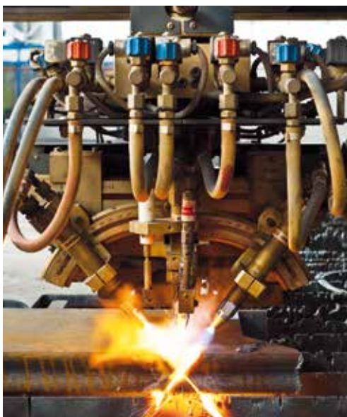
Testa bevel 3 cannelli oxy • 3 torches oxy head
