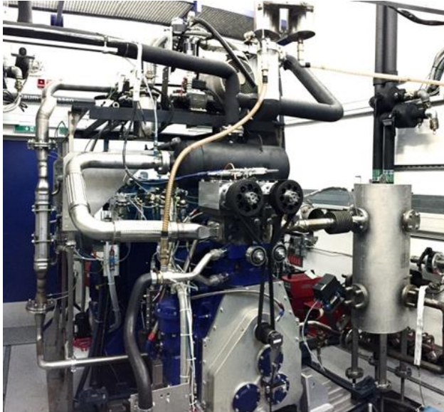
Figure 26 AVL SCE, based on the HDGAS engine [22]
