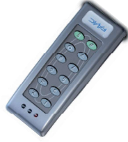
Lettore Key Card e Key Control compatibile con porta blindata Dierre Elettra Key Card and Key Control reader compatible with Dierre Elettra security door
